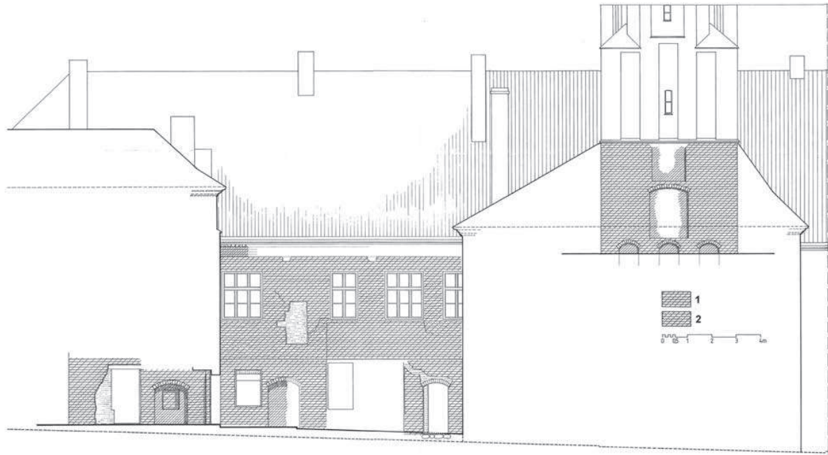
Fig. 11. The east elevation of the middle wing of the town hall and part of the tower with marked examined walls from the 15 th century: 1) original Gothic face, 2) damaged Gothic face (by J. Burnita, S. Kowalski, C. Lasota)
