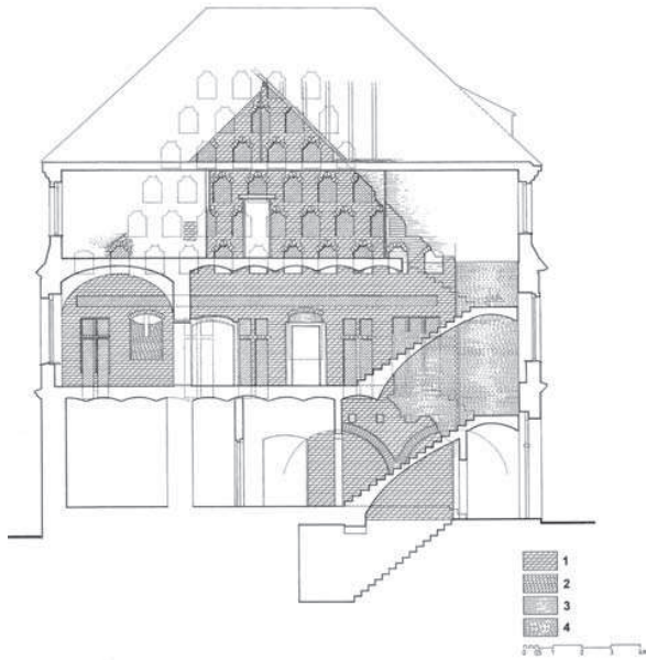
Fig. 7. The north elevation with part of gable of the building of the town hall: 1) wall from the 15 th century, 2) wall from the 1540s, 3) wall from the last third of the 17 th century, 4) wall from 1885–1886 (by J. Burnita, C. Lasota, A. Legendziewicz)
