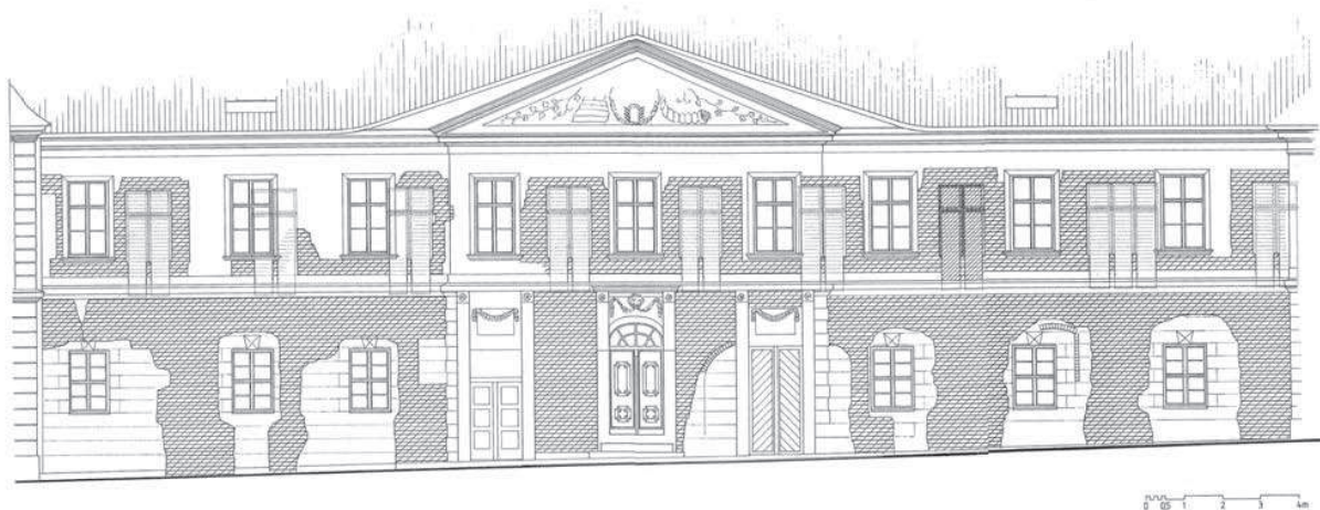
Fig. 9. The west elevation of middle wing of the town hall with the wall from the 15 th century (marked) (by J. Burnita, S. Kowalski)
