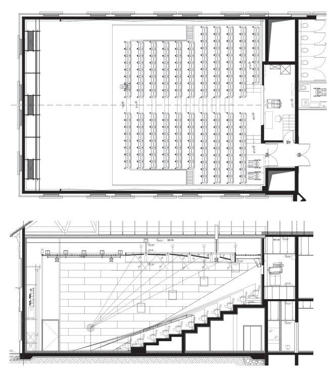
Fig. 1. The Wieliczka Mediateka, performance hall 1<sup>st</sup> floor plan with cross-section, designed by Kozień Architects (source: Kozień Architekci)
