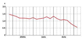
Fig. 5. The Wieliczka Mediateka, reverberation time in the performance hall – performance option without the use of acoustic curtains, designed by Manufaktura Technologiczna (source: Kozień Architekci)
