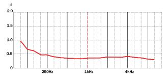
Fig. 4. The Wieliczka Mediateka, reverberation time in the performance hall – cinema option with the use of acoustic curtains (source: Manufaktura Technologiczna)
