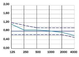
Fig. 8. ICHC Dąbrowa (concert + presentation option), reverberation time with the audience stands set up and acoustic parameter control structures extended (elaborated by J. Rubacha, K. Baruch, K. Brawata)
