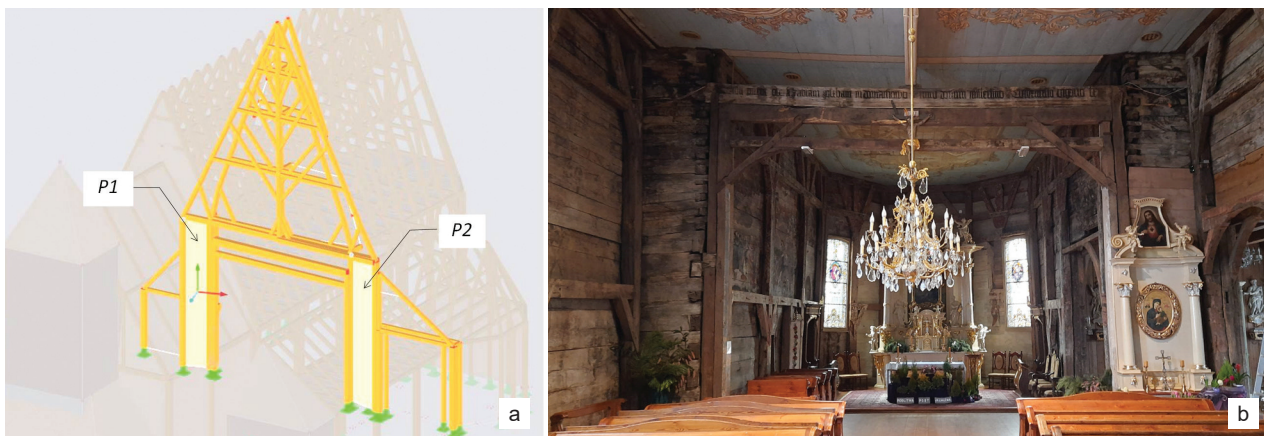
Fig. 8. View of transverse wall at the junction of the nave and the chancel: a) numeric model of the structure – diagram (elaborated by Z. Pawlak), b) view towards the interior of the chancel (photo by Z. Pawlak)
