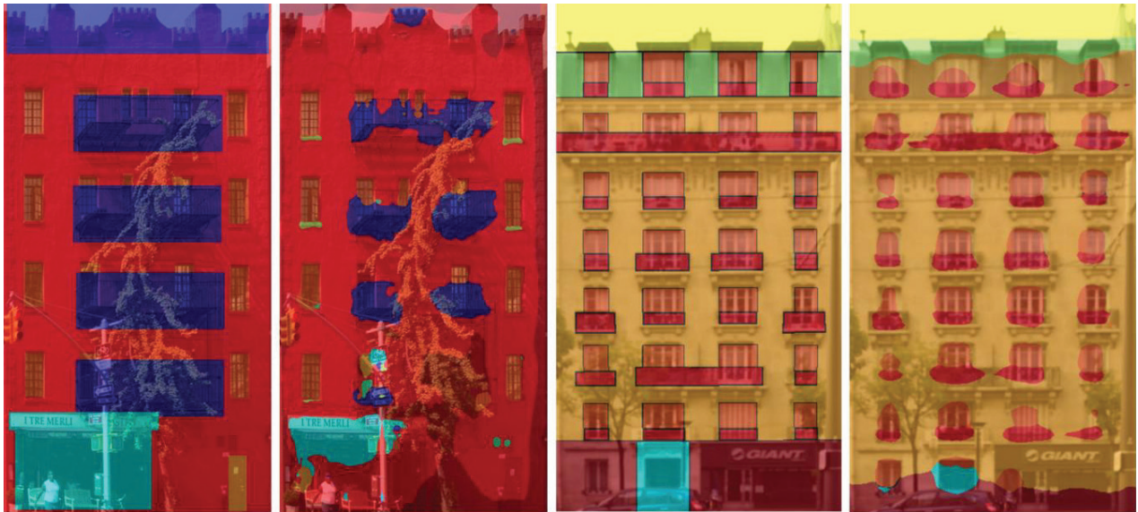
Fig. 2. Ground truth annotations and semantic segmentation results on the CMP dataset (left) and Paris ArtDeco (right) (elaborated by D. Hardzetski)
