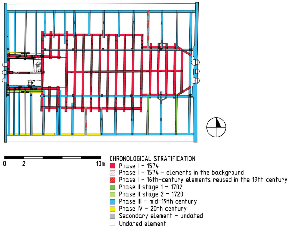
Fig. 3. Church of Our Lady of the Rosary in Byków, chronological stratification of the church, projection at the level of the entablature (elaborated by M. Kumorowicz-Brzeska, U. Schaaf, M. Prarat, D. Jagiełło)
