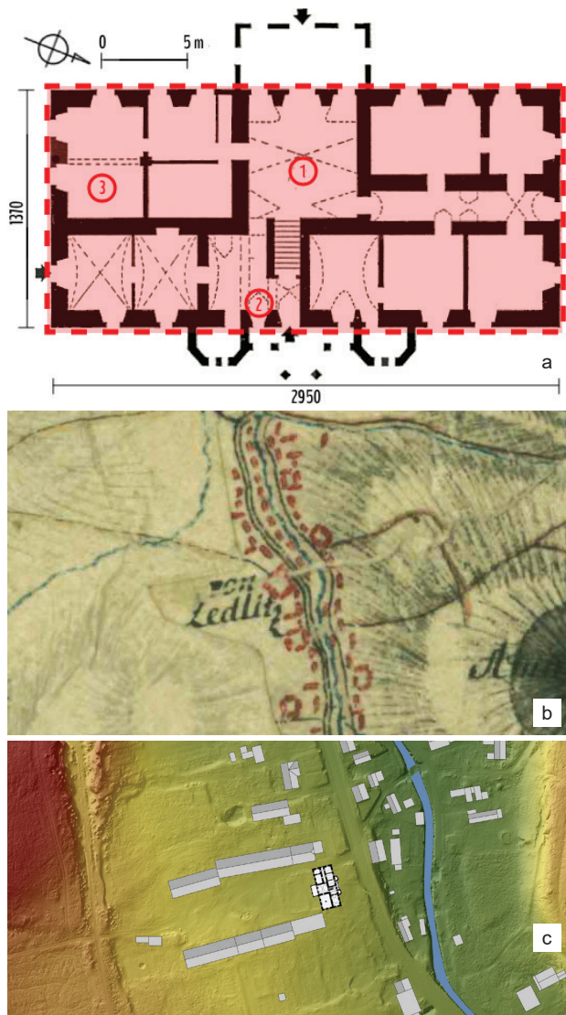
Fig. 7. Niemitz Palace: a) ground plan of the palace, 1 – hallway, 2 – passageway, 3 – probable location of the kitchen (elaborated by A. Walkowska, source: Sawińska, Sawiński 1992a), b) representation of the Niemitz-Kauffung estate on the Regler map (Regler 1763/1770), c) numerical terrain model showing the buildings of the estate (elaborated by A. Walkowska)
