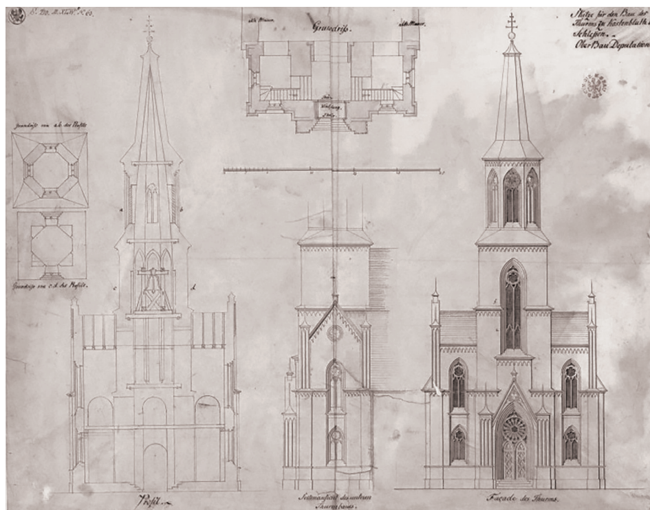
Fig. 6. Design of the tower reconstruction and the addition of staircase annexes according to Schinkel from 1818 (source “Kostenblut (Kostomłoty, ehemals Kreis Neumarkt)...”)
