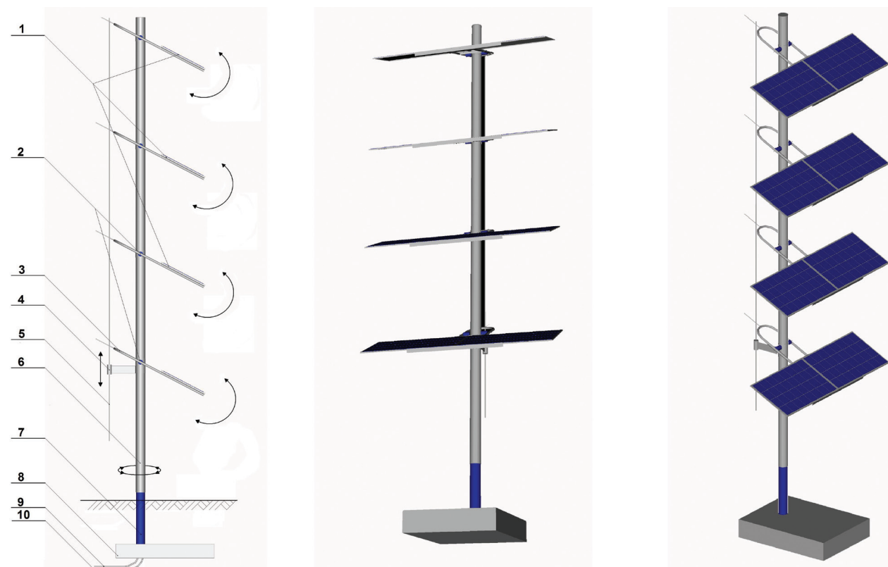
Fig. 9. A proposal for a new type of vertical, rotating, biaxial photovoltaic system solution: a) side view; b) frontal perspective; c) axonometry side.
